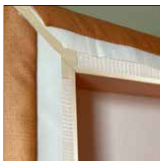
F Fixing the sheet to the frame with strap in the corner
